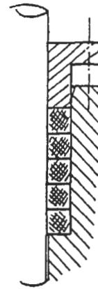
**Figure 25.1 A typical valve stem packing**
