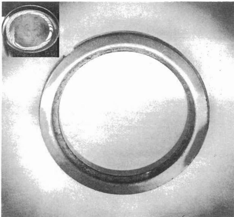
**Figure 6.3 Tungsten carbide mechanical seal face showing localised polishing due to lack of flatness; this seal leaked badly. The inset illustrates a typical non-flat seal face viewed in sodium light using an optical flat to give contour lines at 11 micro-inch increments of height**
