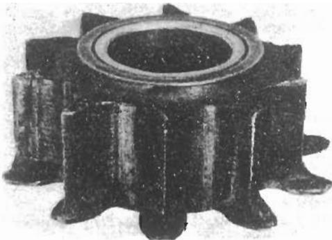
*Spur gear virtually destroyed by foreign matter in the oil*
